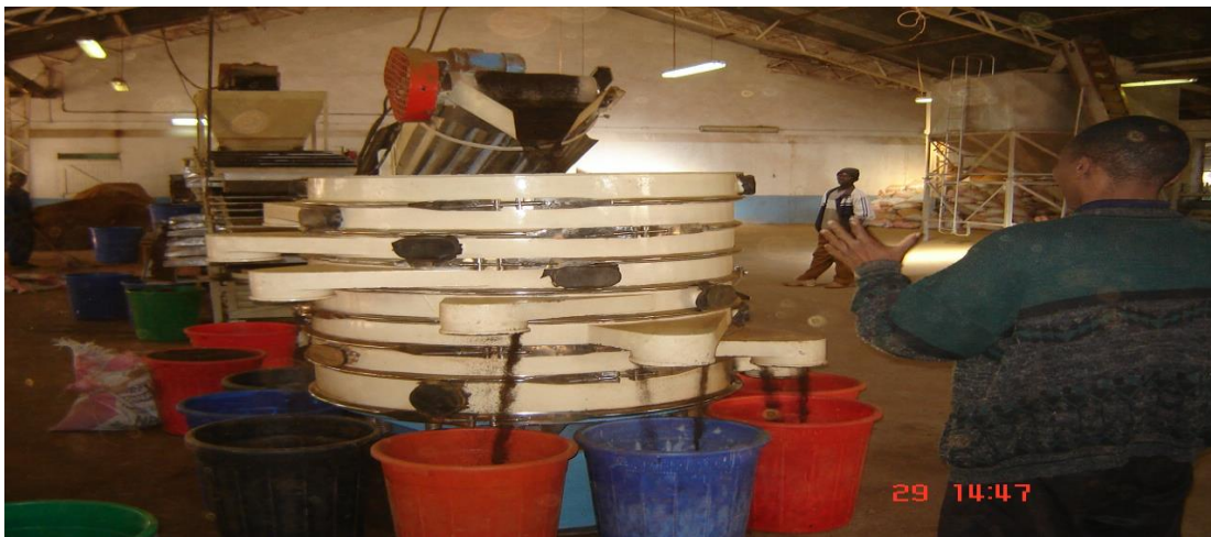
Figure 2.10 Sorting tea - Vibro-Screen Sorter; (Sayama Tea Factory, 2006)
