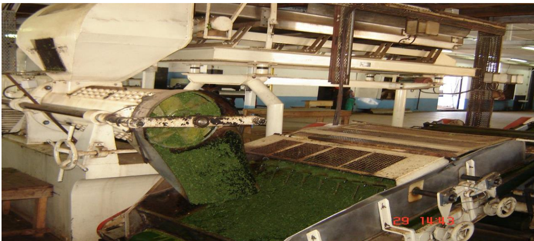
Figure 2.5 Rolling tea using rotorvane/CTC method (Sayama Tea Factory, 2006)
