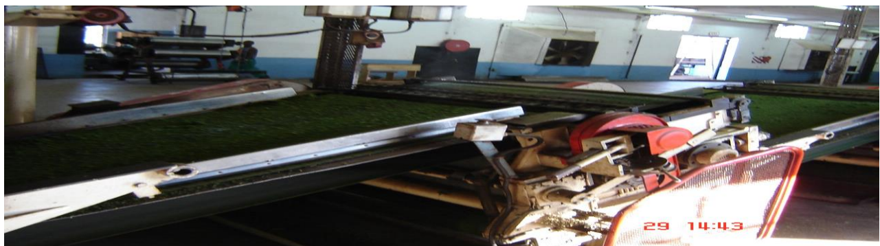
Figure 4.2c CTC Rollers in use (Sayama Tea Factory, May 2006)
