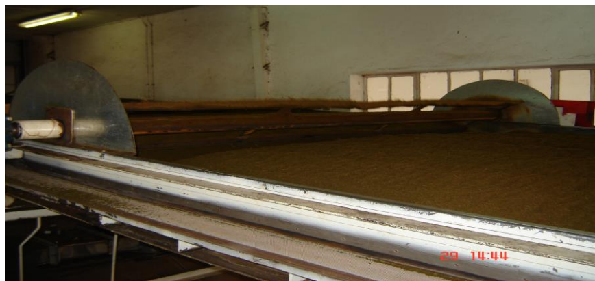
Figure 2.7 Fermenting Tea, leaf changing colour to copper (Sayama Tea Factory, 2006).
