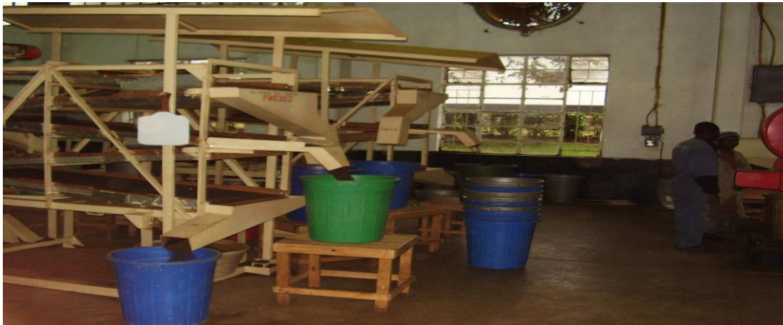
Figure 2.9 Sorting tea - High Speed Sorter (Esperanza Tea Factory, 2006)
