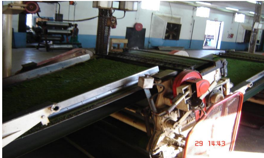
Figure 2.6 Fermenting tea, green leaf at the start of fermentation process (Sayama Tea Factory, 2006).
