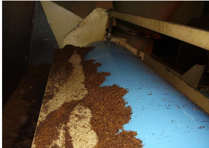
Figure 2.8 Extracting fibres and dust (Esperanza Tea Factory, 2006).
